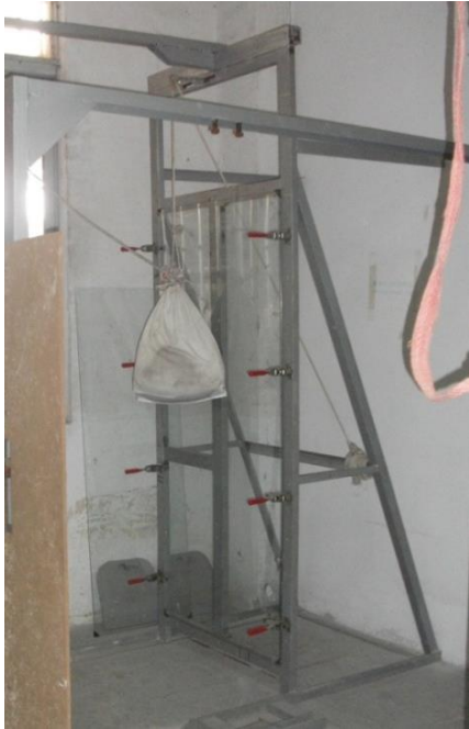
Glass & Shower Room Impact/Load Test
