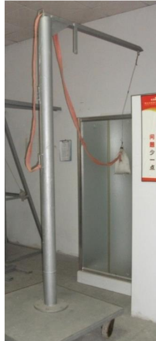
Glass & Shower Room Impact/Load Test
